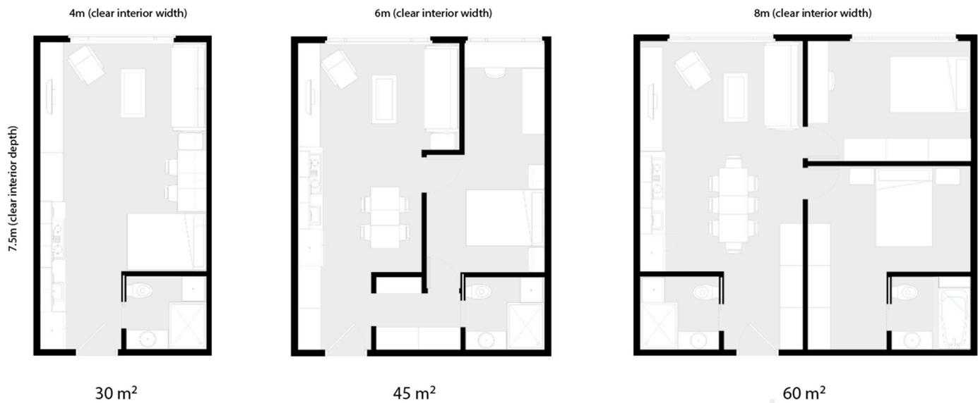
**Figure 2.** Feasible floor plans for one-person, two-person, and three- to four-person minimum floor area units. (Note that for the 60 sqm unit shown here, a second exit door, fire sprinklers, and/or mechanical ventilation would likely be required for code compliance in most jurisdictions.)
