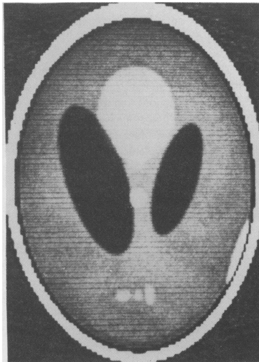
FIG. 4. Reconstruction using the algorithm now embodied in the EMI machine from 180 \times 239 strip projection data obtained by exact calculation from Fig. 1.
