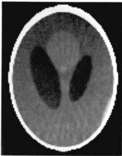
FIG. 18. Reconstruction under same conditions as Fig. 8; plane data m = n = 25 but where the high-contrast out-of-plane objects (eyes, ears, nose, and mouth) have been removed and no longer cast tangents. Compare the quality of this reconstruction with that of Fig. 8. The three small tumors are clearly visible.
